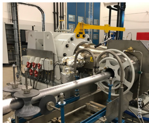
Testing underway on a prototype lead extruder. Used to apply lead sheathing to cables, extruding the metal onto the cables in this way enables longer service life under high stress.
