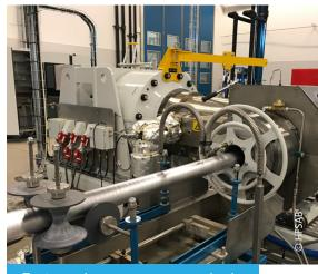
Testing underway on a prototype lead extruder. Used to apply lead sheathing to cables, extruding the metal onto the cables in this way enables longer service life under high stress.
